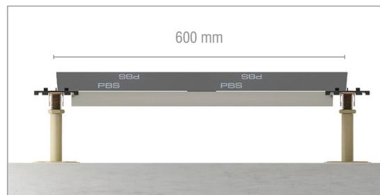
The grid size of pedestal type 2R is 600 mm x 600 mm. Different sizes are possible.
