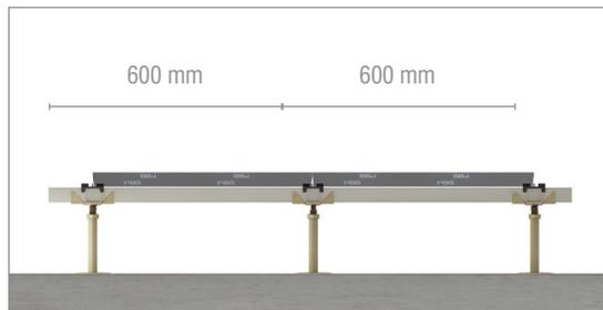
The grid size of this substructure is 600 x 600 mm. Different sizes are possible.
